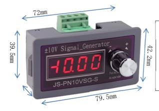
Attention for the installation of cabinet/electric box: The panel must be stuck to the ears on both sides to fix it, so the thickness of the panel must be greater than 1.4 mm, The opening size should consider the width of the ear, and should not be too small, otherwise it will not fit in. The recommended opening size is 77X40mm
